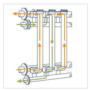
External backwash system shown. Secondary header at the top of the unit introduces cleaning fluid, typically water, (green arrows) to loosen and discharge debris to the drain header at the bottom.
