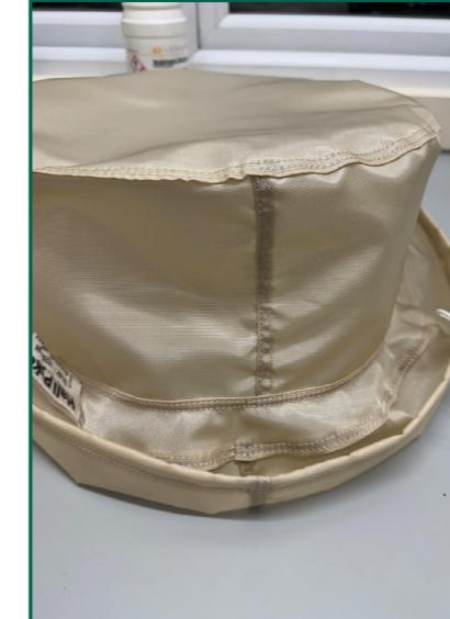
Renowned for its exceptional chemical resistance, mechanical strength, and thermal stability, PEEK is an ideal choice for demanding filtration environments. While Hall Pyke manufactures a wide range of filter bags—from centrifuges to bag filters to leaf filters—across a variety of materials, this marks the first time the company has produced a solution specifically for use with a Buchner Funnel.
